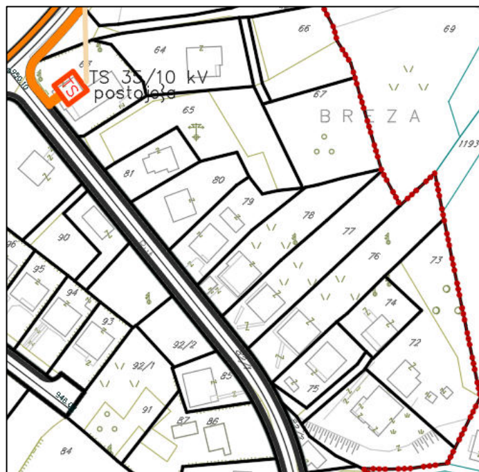
novoplanirana TS 10/0.4kV/kV planirani 35kV- kabal
